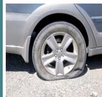
Driving on a flat tyre can cause the rim to ride on the tyre tread or the ground potentially resulting in loss of control of the vehicle .
