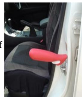
To break the windows, a metal tip has been installed and a cutter in the handle which will cut the seat belt if ever there is a buckle malfunction.
