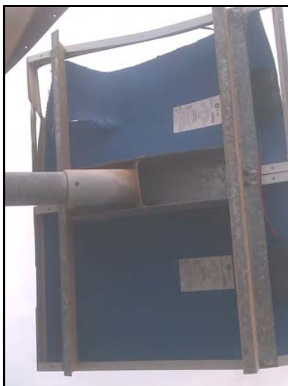
Pictured left is the reverse side of solar panel where the panels and components have been removed.
